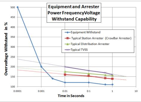
Figure 3 Overload Speed of Arresters and Withstand of Equipment
